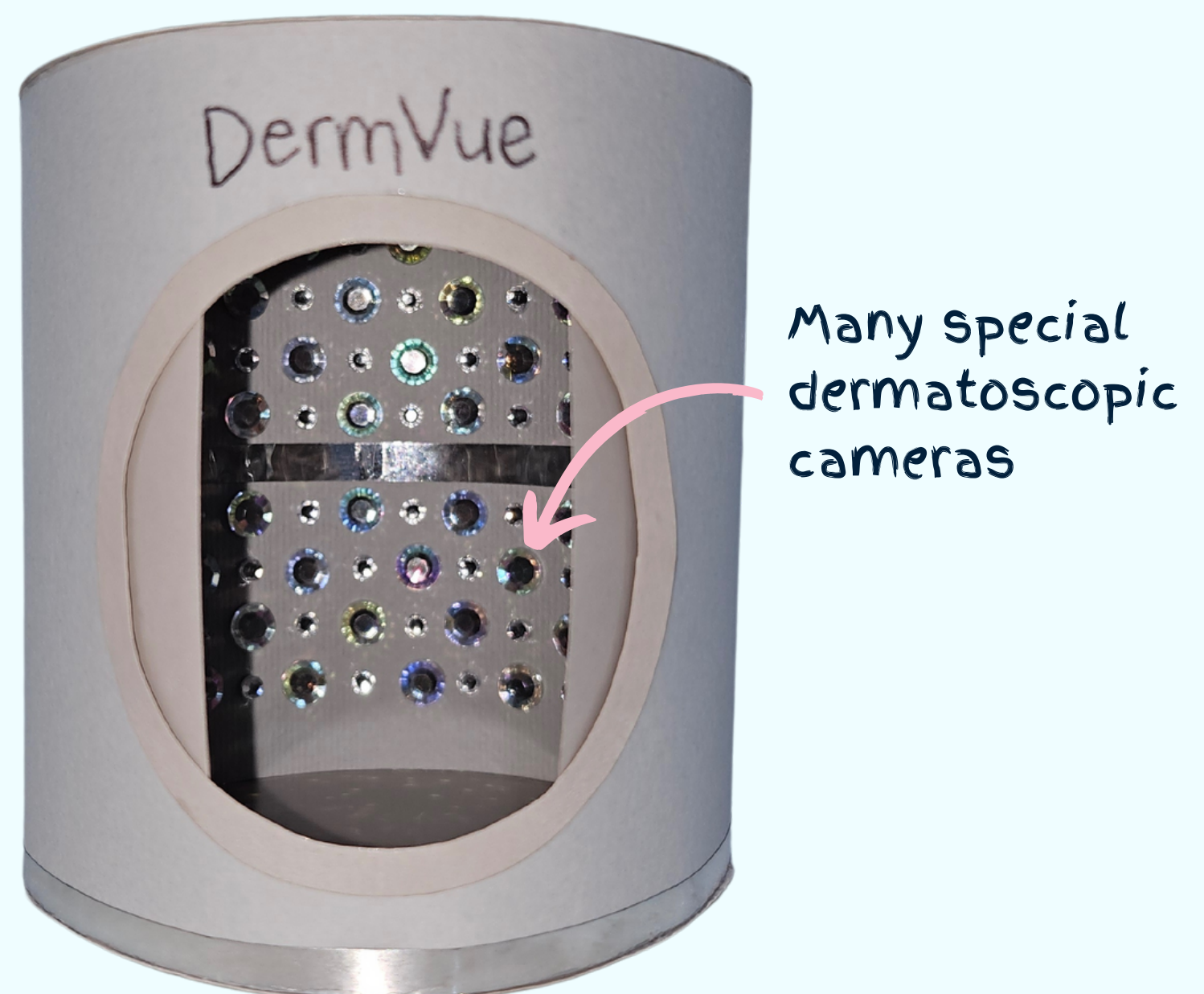
Photo 2. Real-life prototype of DermVue
